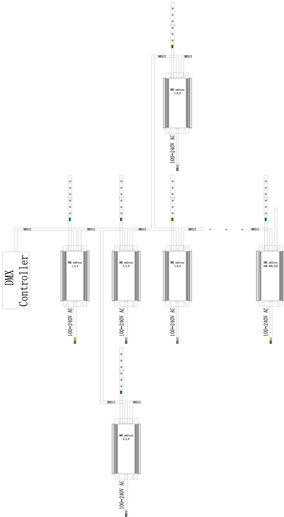
DMX connection for RGB (fig.9)
