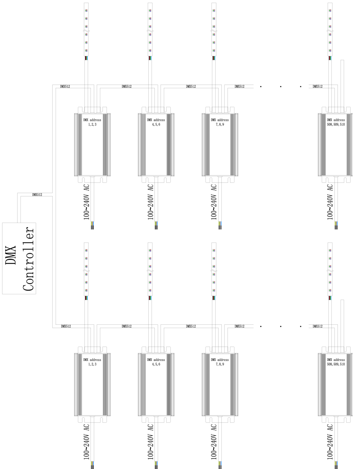
DMX connection for RGB (fig.7)
